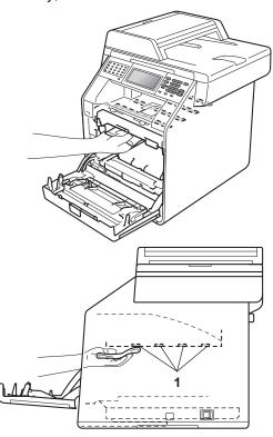
6 Make sure the green lock lever (1) is in the release position as shown in the illustration.
